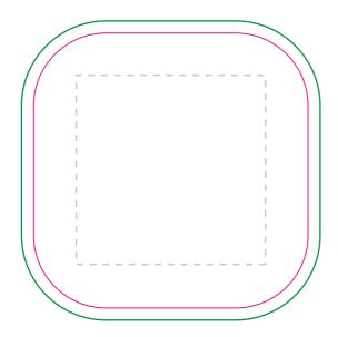
Dotted line indicates maximum Pad print area Pink line indicates Digital insert cut area Green line indicated bleed area reaguired for Digital insert
