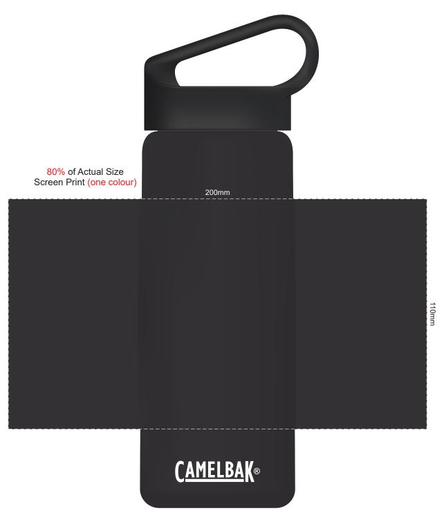
A 2-3mm tolerance is expected for alignment of the printed artwork and the CamelBak logo.
